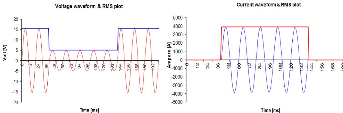
Figure 4.7 Downstream fault current causes voltage sag in the network
