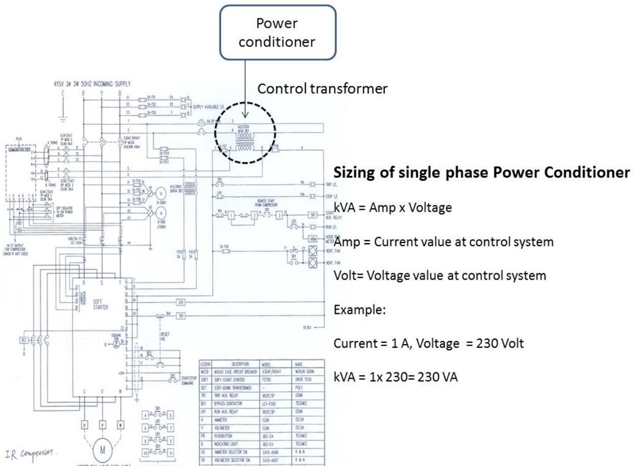
**Note.** Please ensure there is no undervoltage relay (UVR) at the control circuit.
