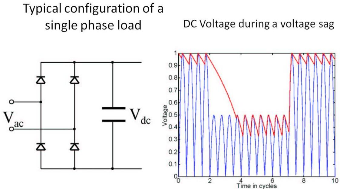
Figure 4.29 The resultant dc voltage during a voltage sag event
