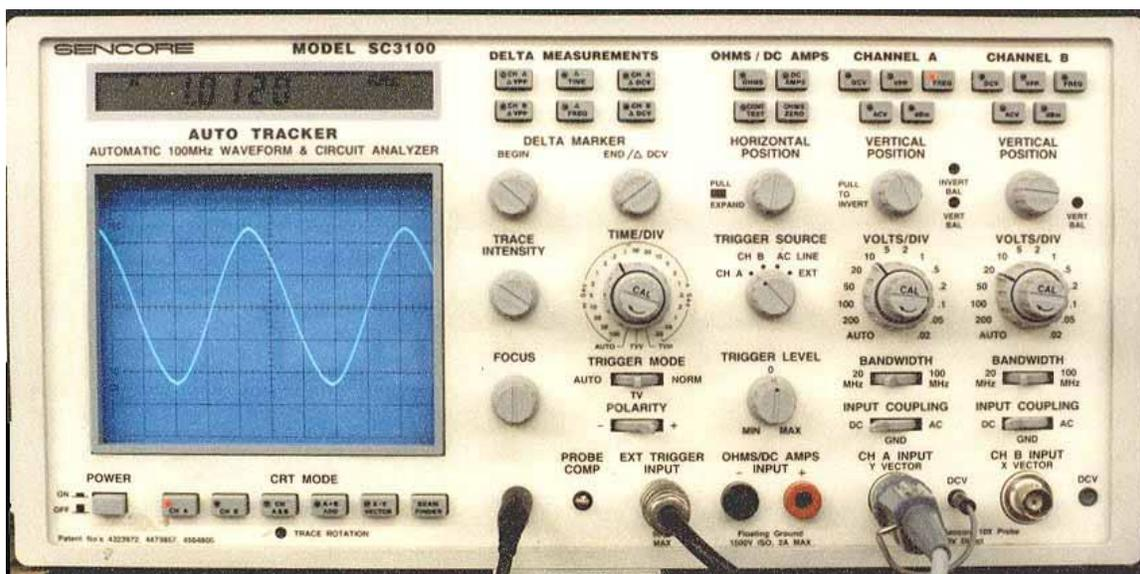
Figure 5.1 Oscilloscope: Image of an ac voltage sine wave
