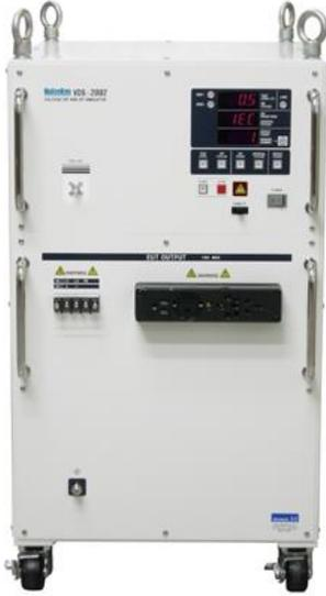
Figure 7.6 Voltage Dip & Swell Simulator VDS 2002
