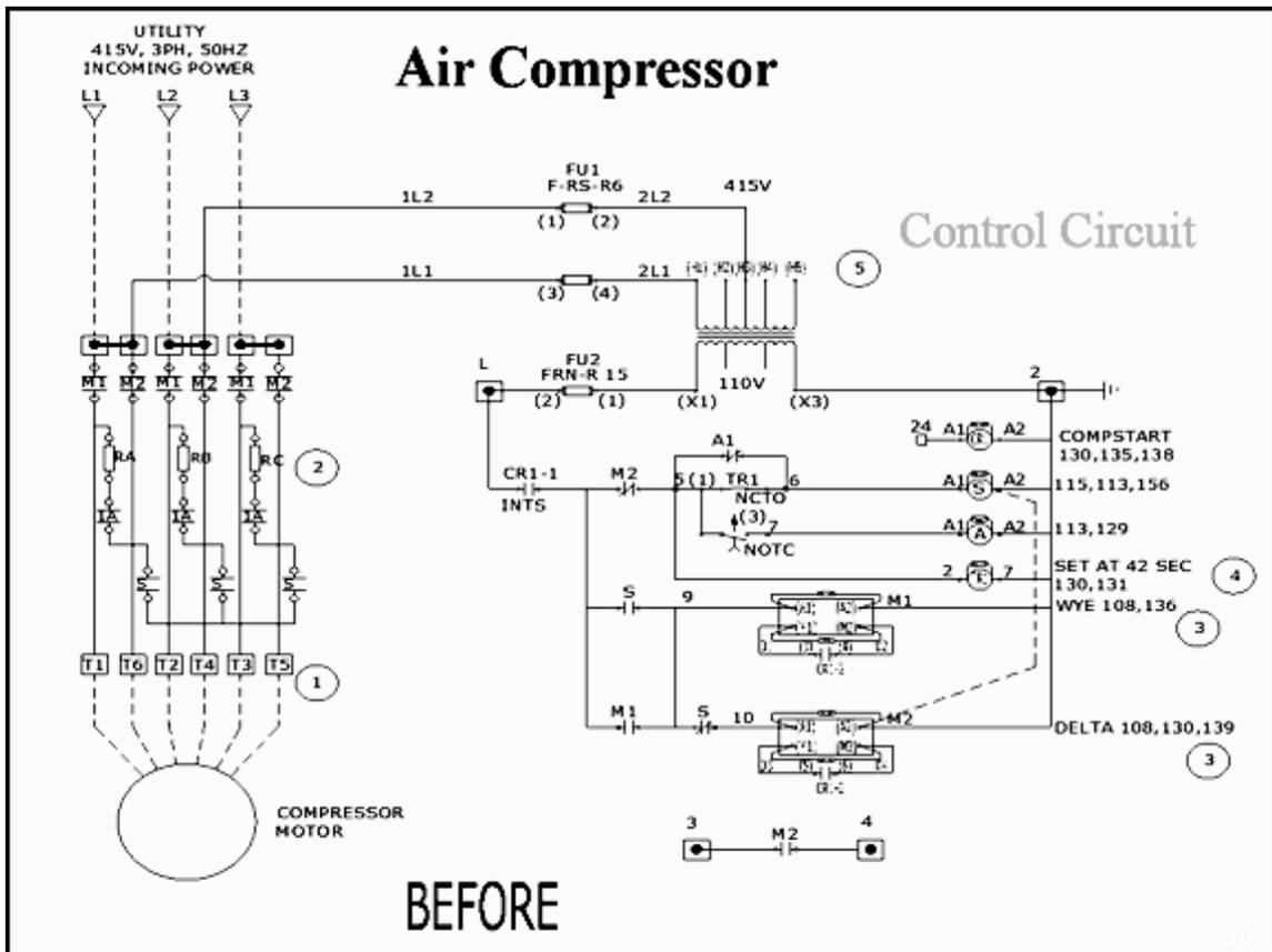
Figure 4.28 General circuit for control circuit & contactor (2)
