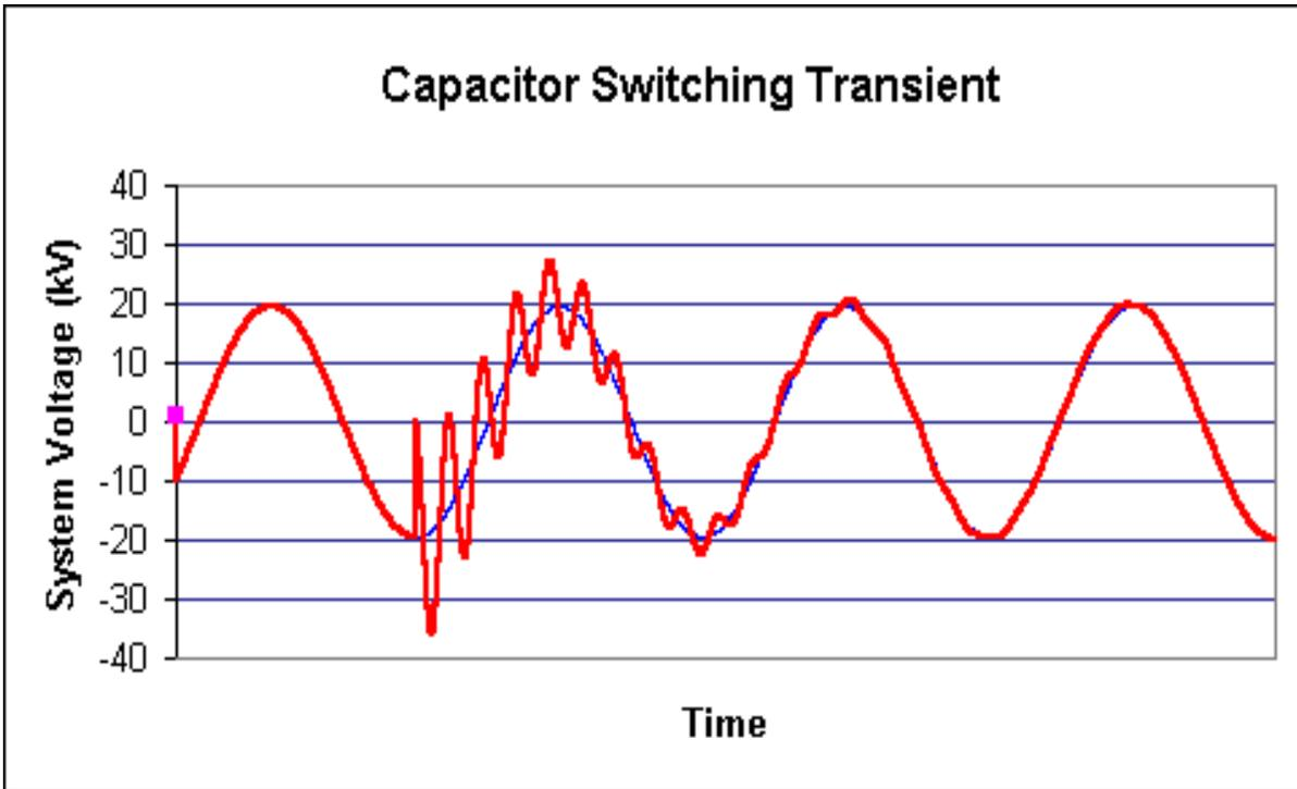
Figure 5.5 Oscillatory Transient due to capacitor switching
