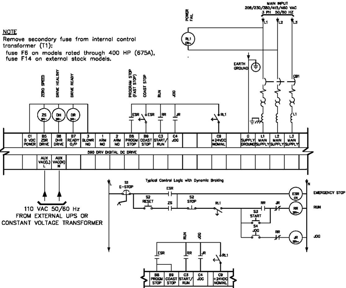
Figure 4.32 Control power to a 590 Drive for Power Loss Ride Through
