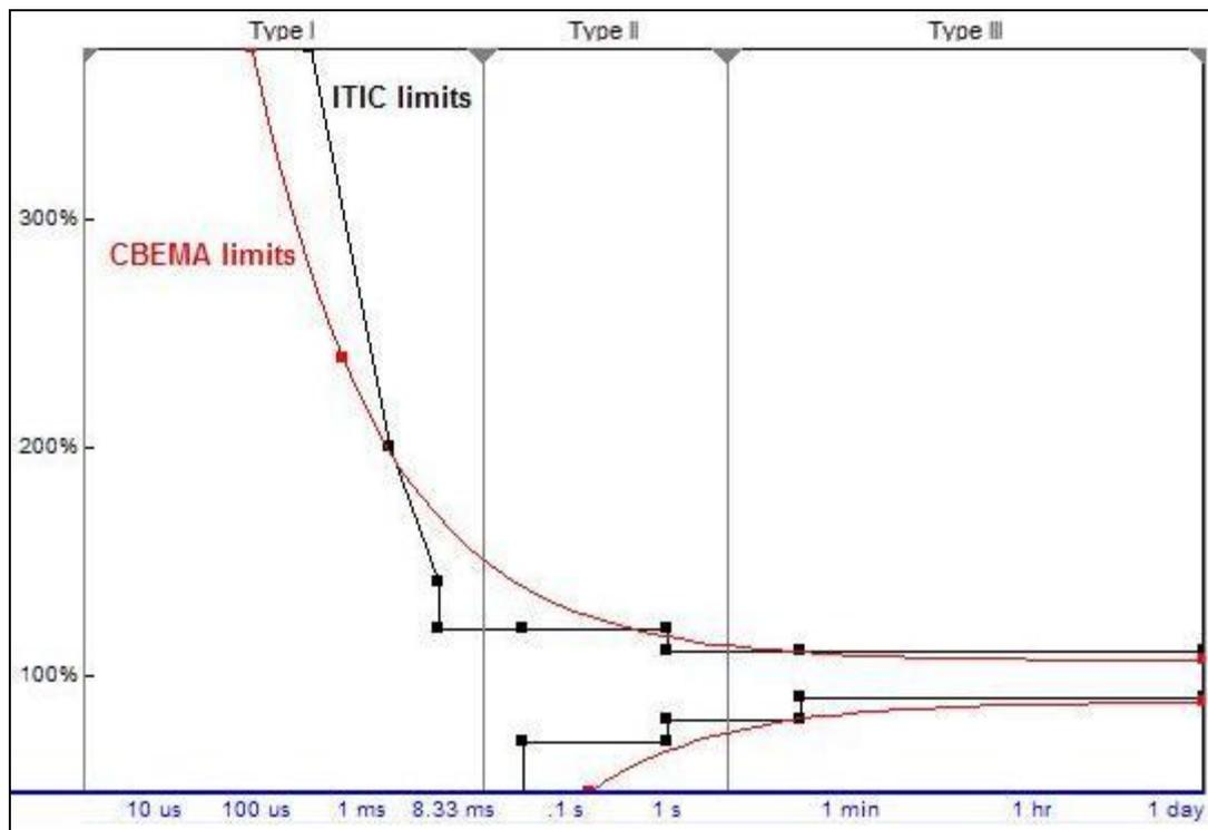
Figure 6.2 ITIC & CBEMA curve
