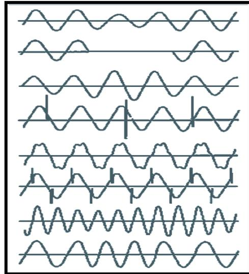
Waveforms recorded by a power quality recorder
