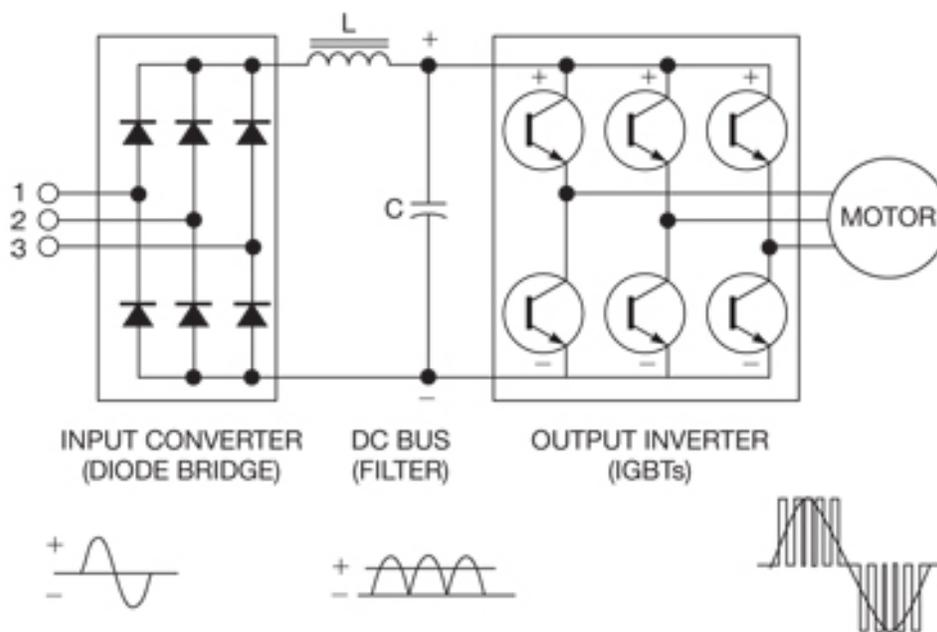
Figure 8.6 Single line diagram for a typical Adjustable Speed Drive (ASD)
