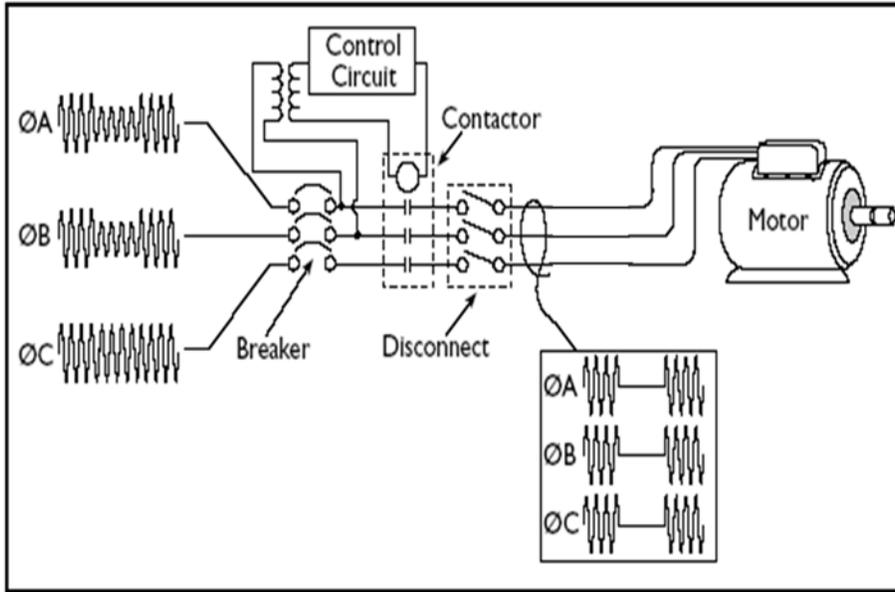
Figure 4.27 General circuit for control circuit & contactor (1)
