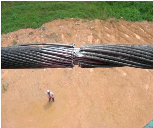
Conductor damaged due to a kite
