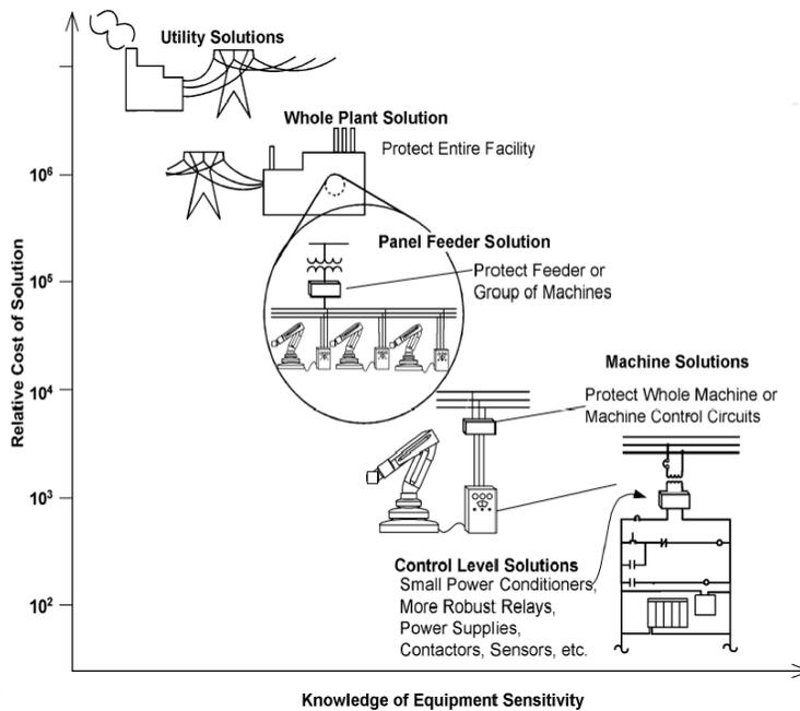
Figure 8.9 Level of equipment sensitivity and cost of solutions
