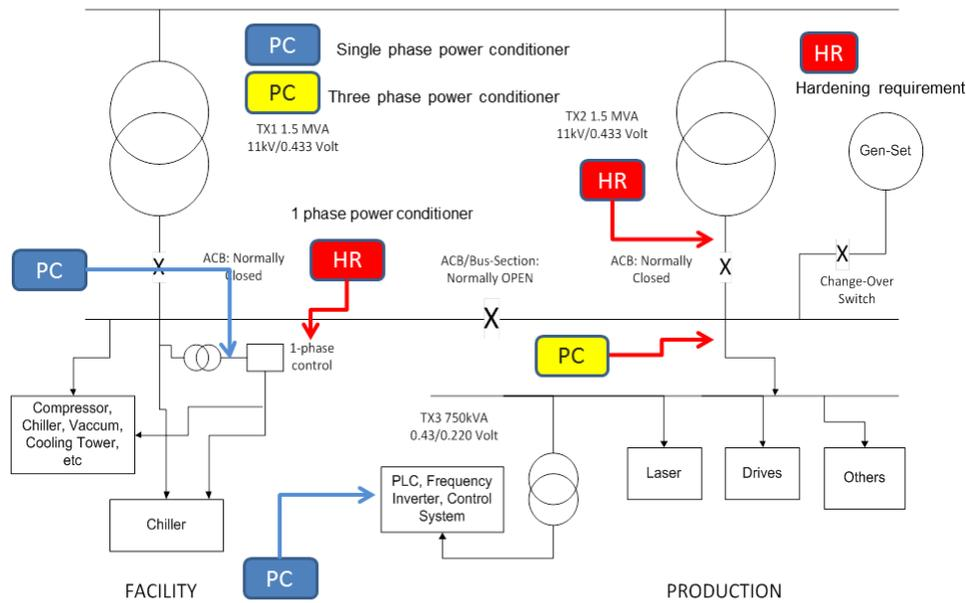
Figure 10.1 Location to implement mitigation action to improve the immunity of the critical process and equipment against voltage sags.
