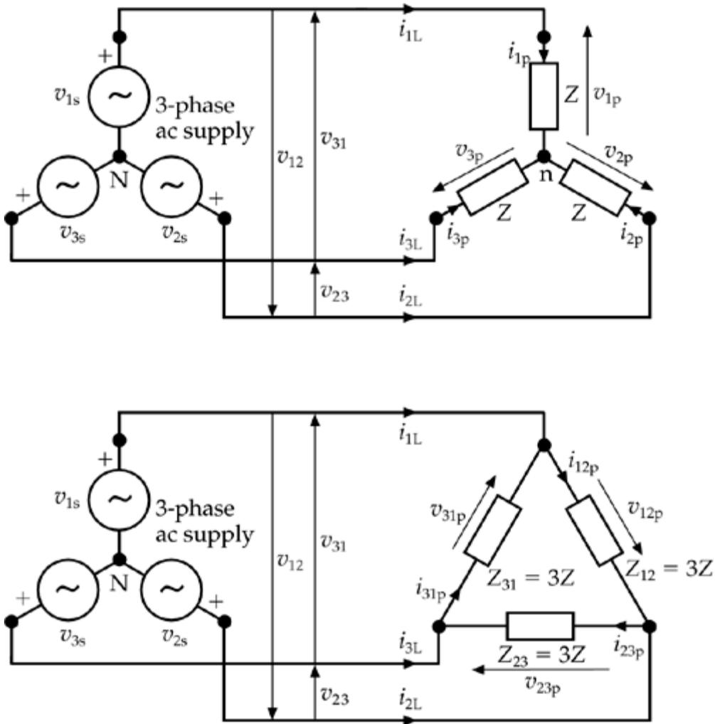
Figure 4.18 Star & Delta connections of three phase loads
