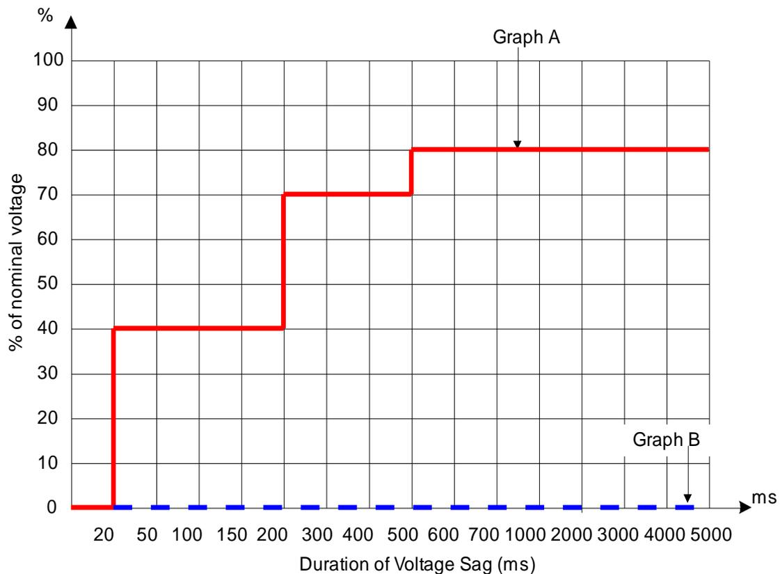
Figure 6.5 IEC 61000-4-34 (Class 3) curve
