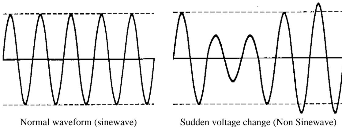
Figure 4.1 Normal waveform and power quality waveform (voltage sag)
