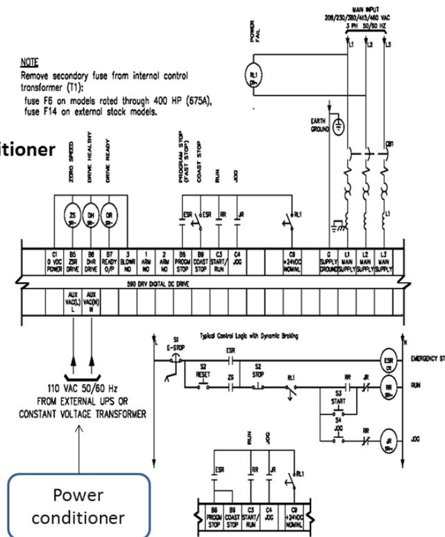
**Note.** Please ensure there is no undervoltage relay (UVR) at the control circuit.
