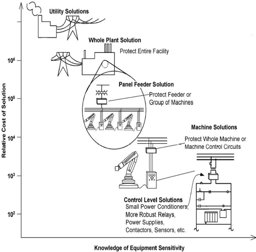
From Figure 8.9 Level of equipment sensitivity and cost of solutions
