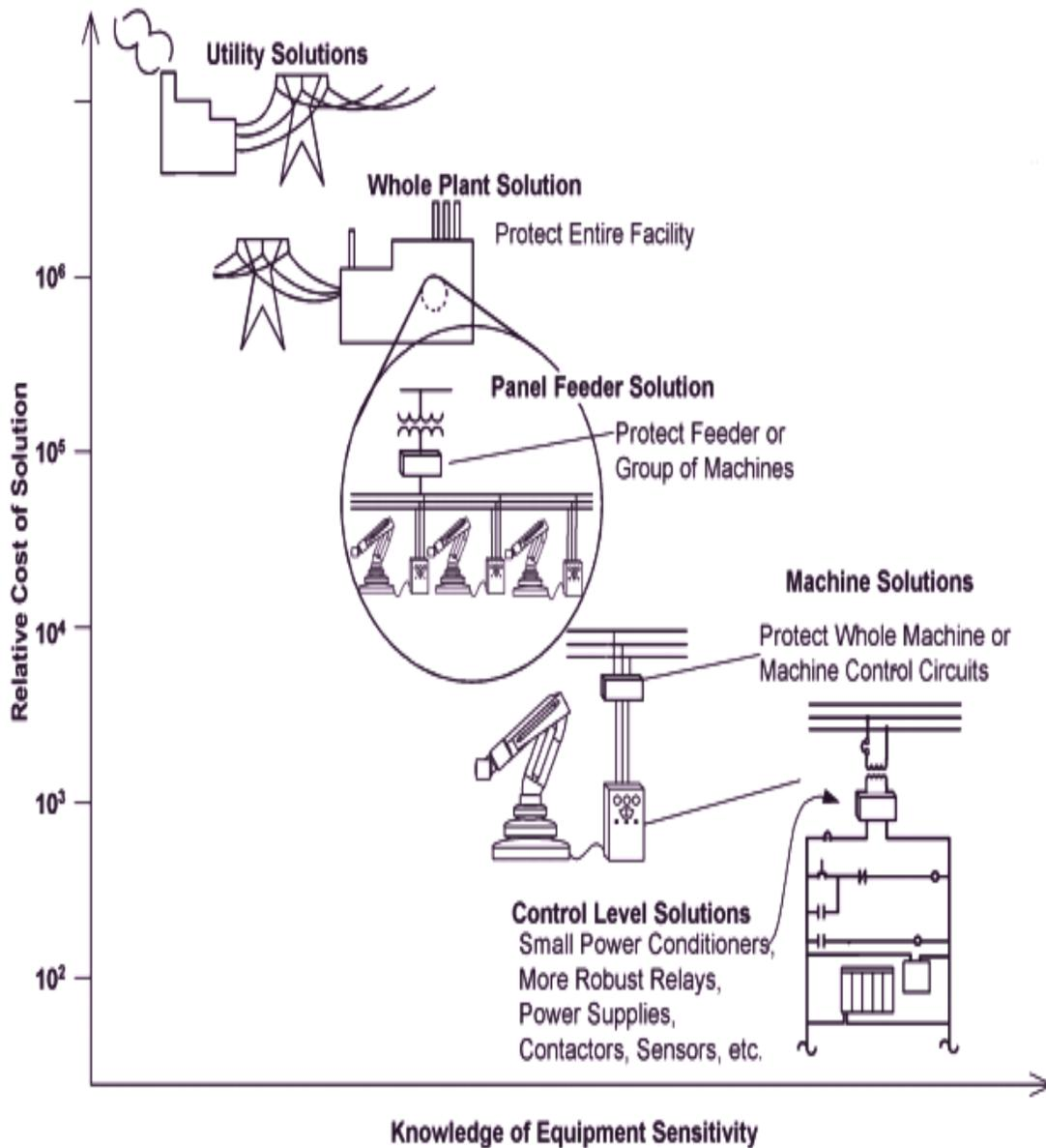
Figure 4.22 Levels of equipment sensitivity & cost of solutions [17]
