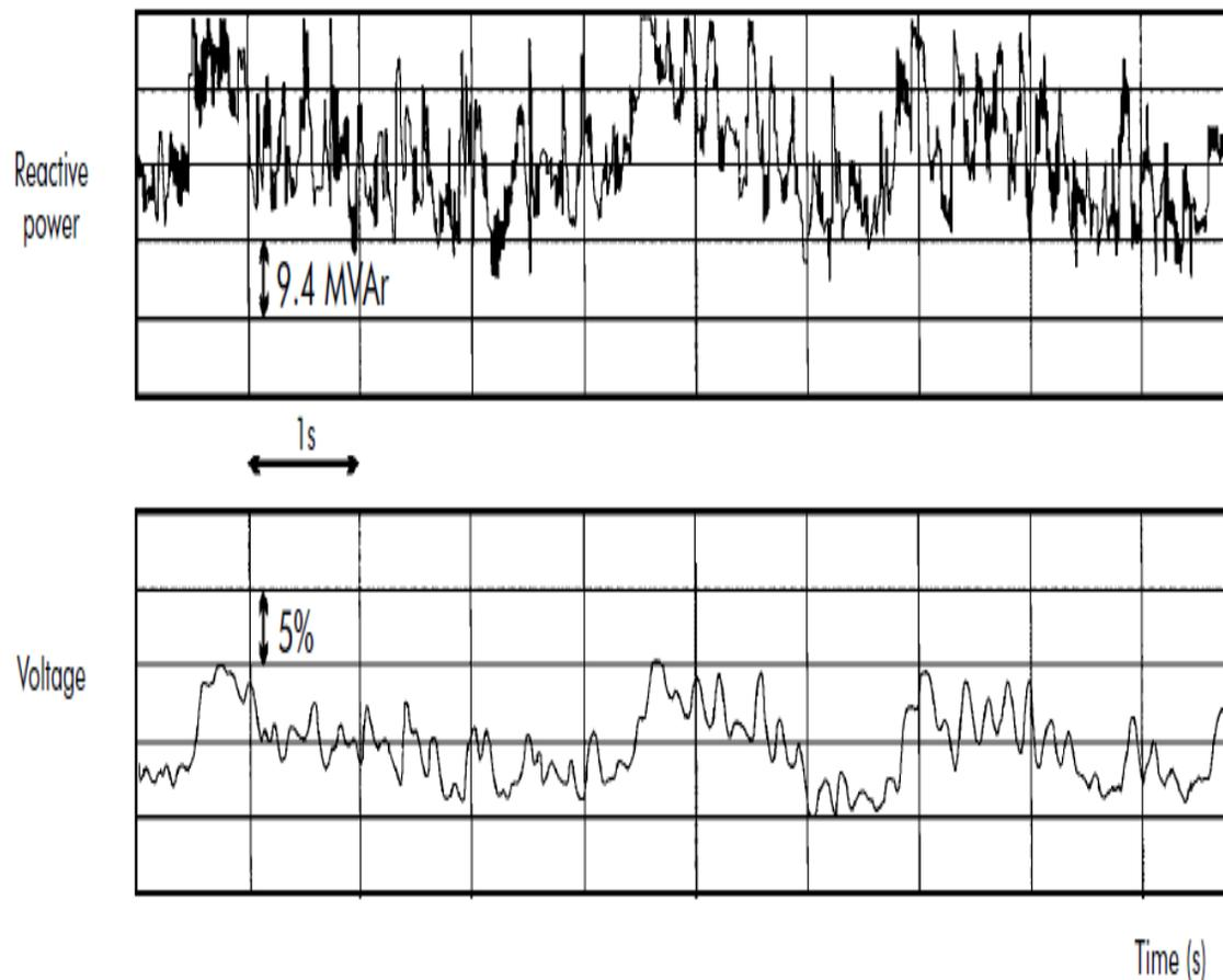
Figure 5.2 Changes in the reactive power and the resulting voltage fluctuations at the point of connection of an arc furnace
