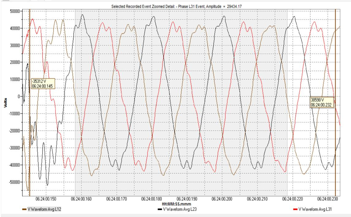
Figure 5.3 Harmonics waveforms recorded in a steel mill
