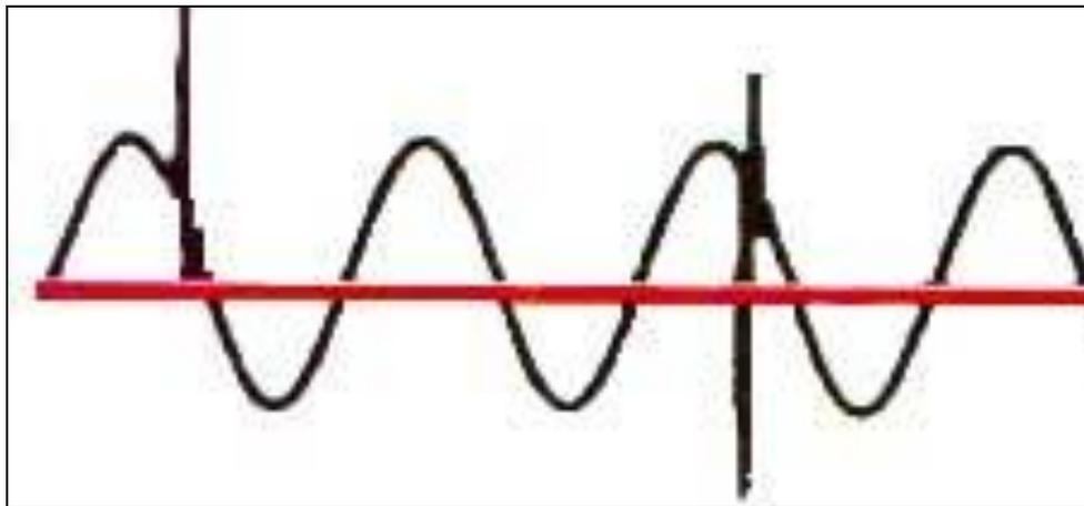
Figure 5.6 Waveform due to Impulsive Transient
