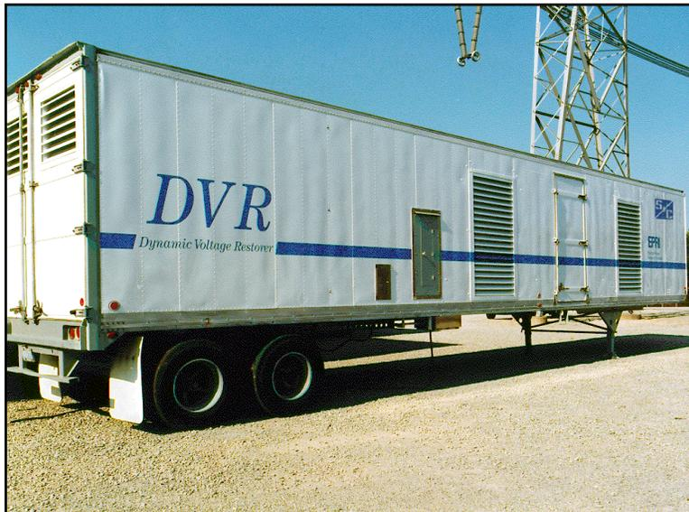
Figure 9.7 Dynamic Voltage Restorer
