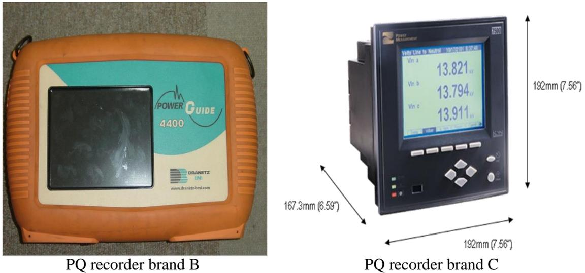
Figure 5.7 Examples of PQ recorders
