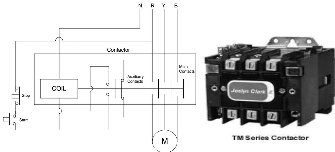
Figure 4.26 A common contactor
