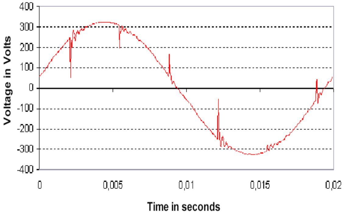
Figure 5.4 Notches voltage waveform
