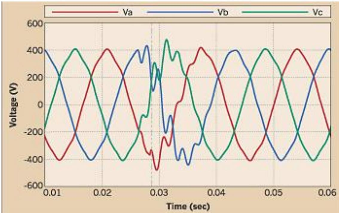
Figure 5.7 Multiple PQ disturbances (Oscillatory Transient & Harmonics)
