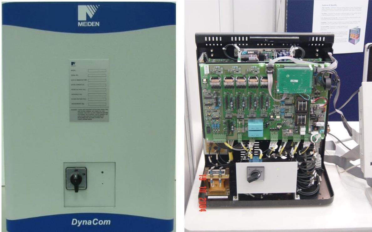
Figure 8.16 Dynamic Compensator (Dynacom)
