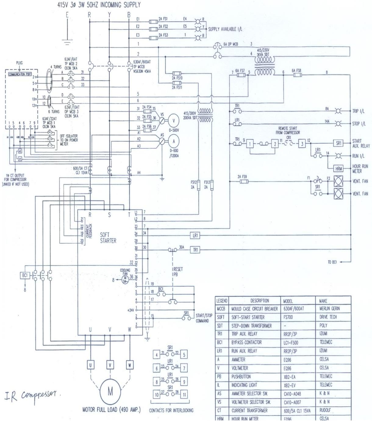
Figure 4.33 Diagrams for control circuits for compressor
