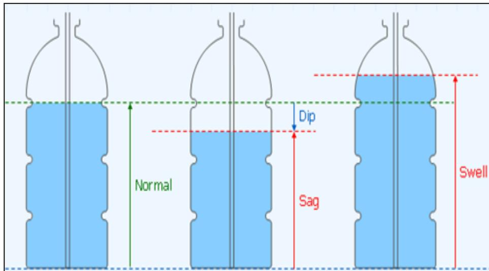
Figure 4.6 Graphic definitions of normal voltage, dip, sag and swell
