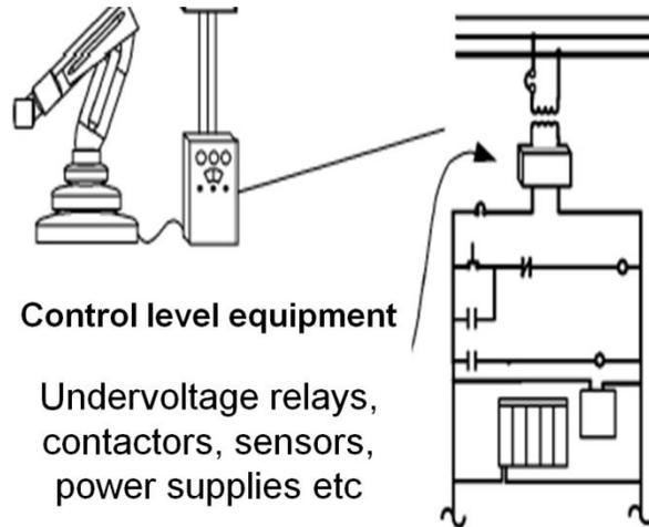
Figure 4.23 General control level equipment & solutions
