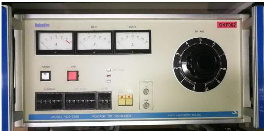
Figure 7.8 Voltage Dip Simulator VDS-220B
