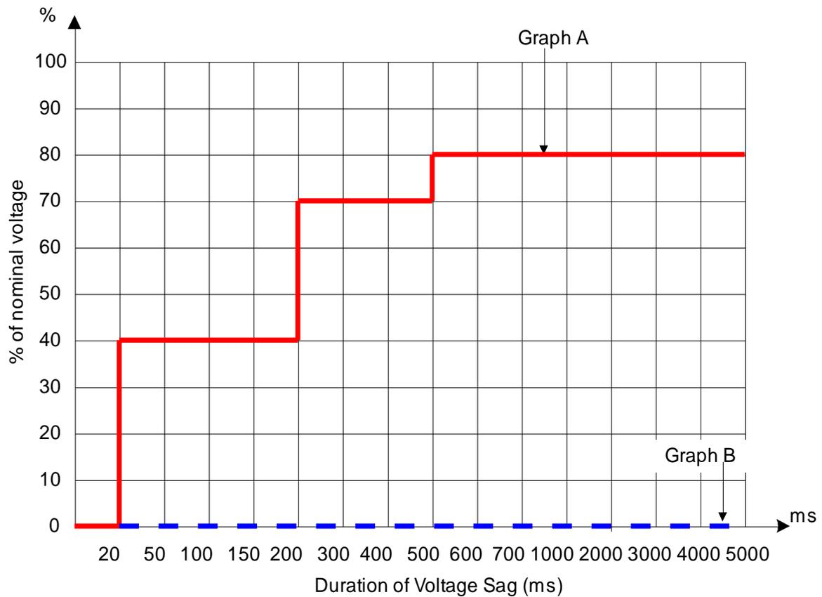
Figure 6.4 IEC 61000-4-11 (Class 3) curve
