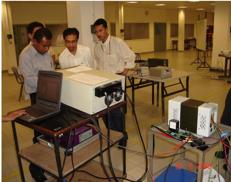
Figure 7.10 Voltage tolerance testings using IPC & Chroma equipment
