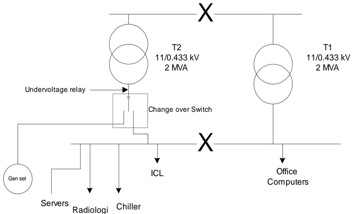
Figure 4.25 Common locations for under voltage relay (UVR)
